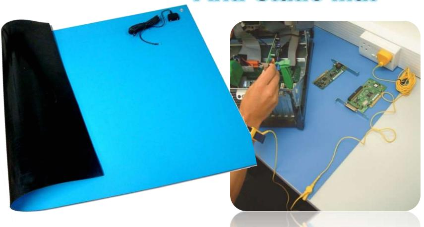
used to **stand on** or **place hardware on** to prevent static electricity from building up.
