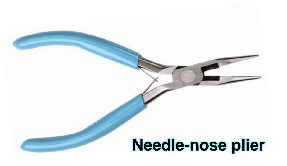
used to **hold** small parts.
